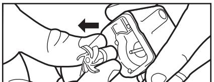
**EN** Open the pump, remove the impeller cap and impeller.
