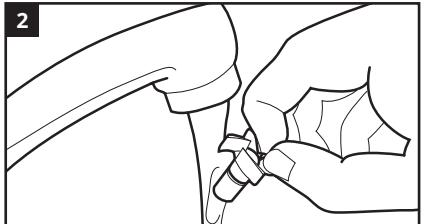
**EN** Rinse each part with water, removing any hairs or debris from the impeller and pump housing, before carefully reassembling.
